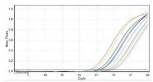
Most relevant HCV genotypes (1-2-3-4-5) were tested analyzing dilution series and results showed good and clear sigmoid-shaped fluorescence curves and a Cycle threshold (Ct) less than 35.
