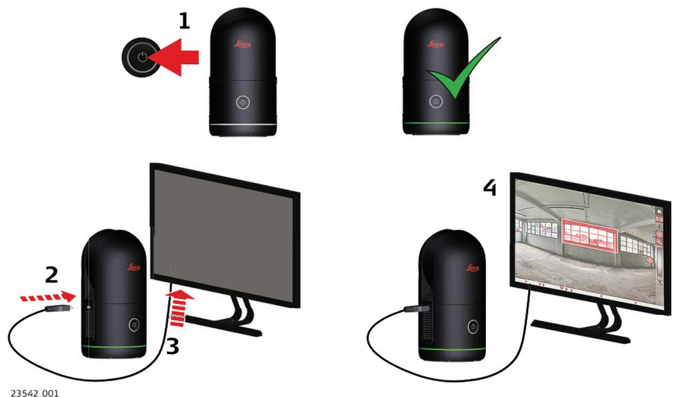
1. It is recommended to start the BLK360 first to ensure the fastest data transfer.
