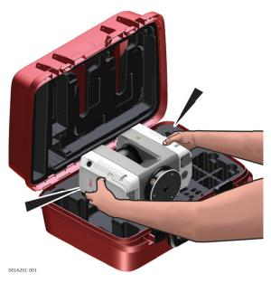
To take the instrument out of its container, grasp the instrument at the left and right side covers, and lift.
