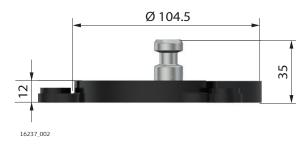
GAD122 adapter to mount a RTC360 on top of a Leica tripod:
