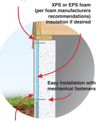
Durable rubberized covering with resilient white foam backing resists damage from projectiles due to lawn mowing etc.
