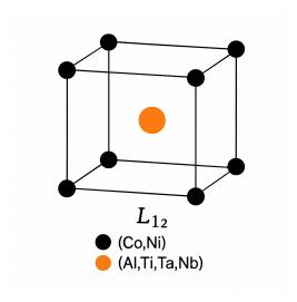
The ordered nature of  $L1_2$  causes significant strengthening because the  $\gamma'$  precipitates resist dislocation movement through coherency strains and anti-phase boundary formation. This is fundamental in high-temperature applications such as gas turbines, reformers, petrochemical reactors, and other components requiring long-term creep resistance.
