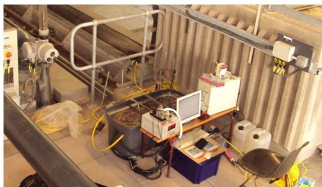
Fig. 3 Photograph of the reactor in situ at Howden wastewater treatment site
