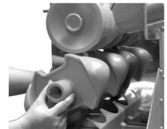
Remove the squeezer drum by unscrewing the screw. Remove the second squeezer male part.
