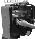
Remove the front cover, by unscrewing the two lateral screws.
