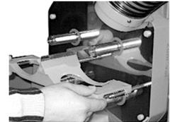
**For the models with the upper feeder component,** twist softly the upper metal basket all the way towards the left and then gently pull up. Remove the turning dish by unscrewing the screw towards the right.
