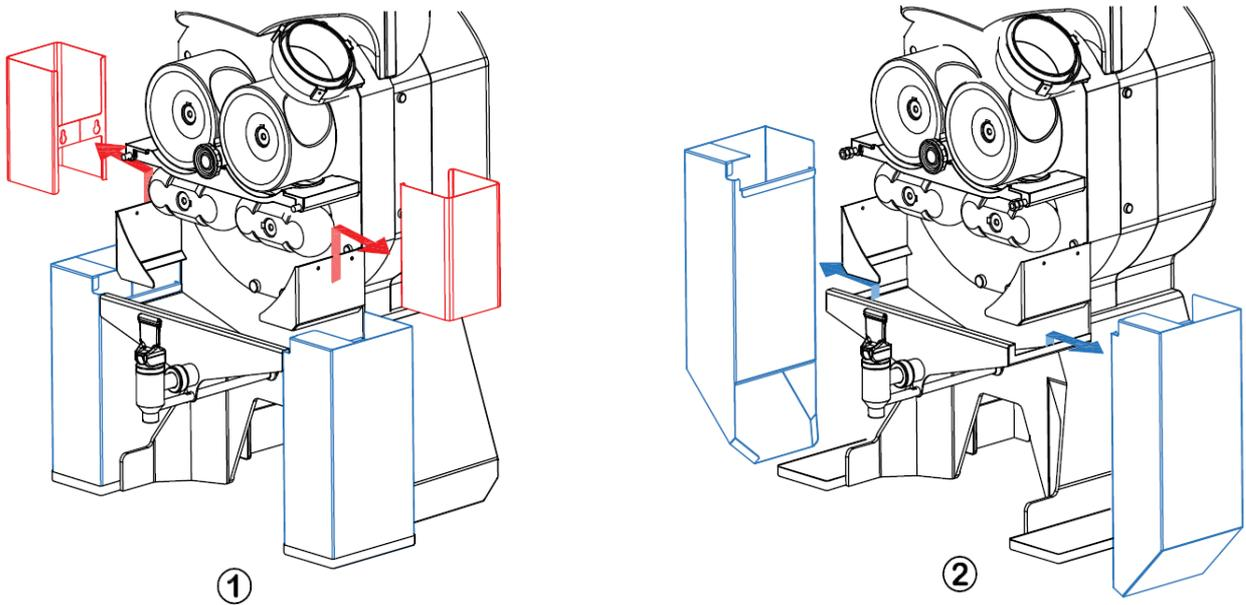
1. Once front cover has been removed, remove top squared tubes by displacing, first, vertically and, second, horizontally.
