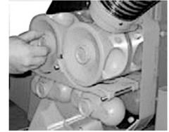
Remove the two squeezing drums, the two male parts and knifepiece pulling it outwards. Be careful with this part, because of its cutting edge.
