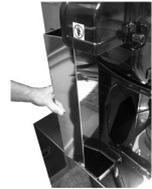
Remove the front cover, moving it slowly upwards and towards.
