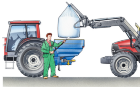
Use a knife with a long handle to cut the bag. Never walk under suspended load!
