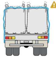
Check lashing tensions
