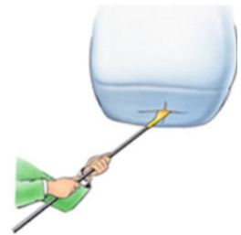
The bulk bag is emptied by two crossed incision in the middle of the underside of the bag (30-40 cm).
