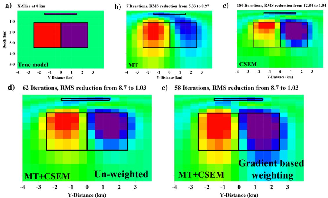
**Figure 1:** Results obtained from inverting MT and CSEM data separately and jointly. The true 3-D model consists of a shallow and thin resistive block and two deeper conductive and resistive blocks. For the joint inversion results we applied our proposed gradient based weighting scheme.
