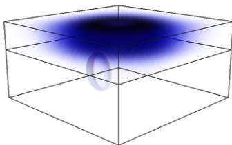
**Figure 5.** Normalized current densities of the layered half-space model with conductive structure at  $t \approx 3.2 \times 10^{-4}$  s. One can nicely see that the conductive structure starts to “capture” the electric currents.
