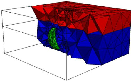
**Figure 4.** Cut of the coarsest mesh of the layered half-space model with conductive structure. The overburden is shown in red, the underlying half-space in blue and the herein embedded conductive structure in green.
