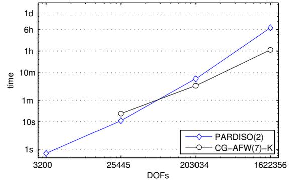
**Figure 2.** Computation times for the homogeneous half-space model for different grid sizes (identified by different number of degrees of freedom on the  $x$ -axis). The direct sparse solver PARDISO is compared to CG with multigrid as preconditioner.
