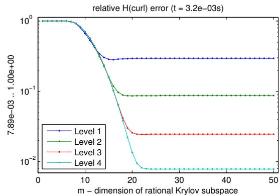
**Figure 3.** Convergence behavior of the rational Krylov subspace method for fixed time and varying dimension of the subspace. “Level” refers to the different meshes of increasing fineness.
