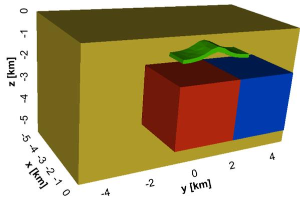
Figure 1: Synthetic model for the Multi-EM project, currently used in Freiberg for DC inversion with  $\sigma_1 = 0.1 \frac{\text{S}}{\text{m}}$  (yellow),  $\sigma_2 = 0.01 \frac{\text{S}}{\text{m}}$  (green),  $\sigma_3 = 1 \frac{\text{S}}{\text{m}}$  (red) and  $\sigma_4 = 0.002 \frac{\text{S}}{\text{m}}$  (blue).
