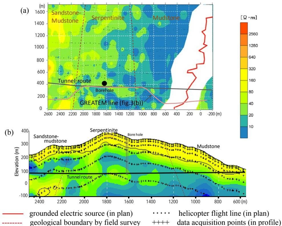
**Figure 3.** Electrical resistivity slice of depth 300 m (a) and profile of tunnel line (b).
