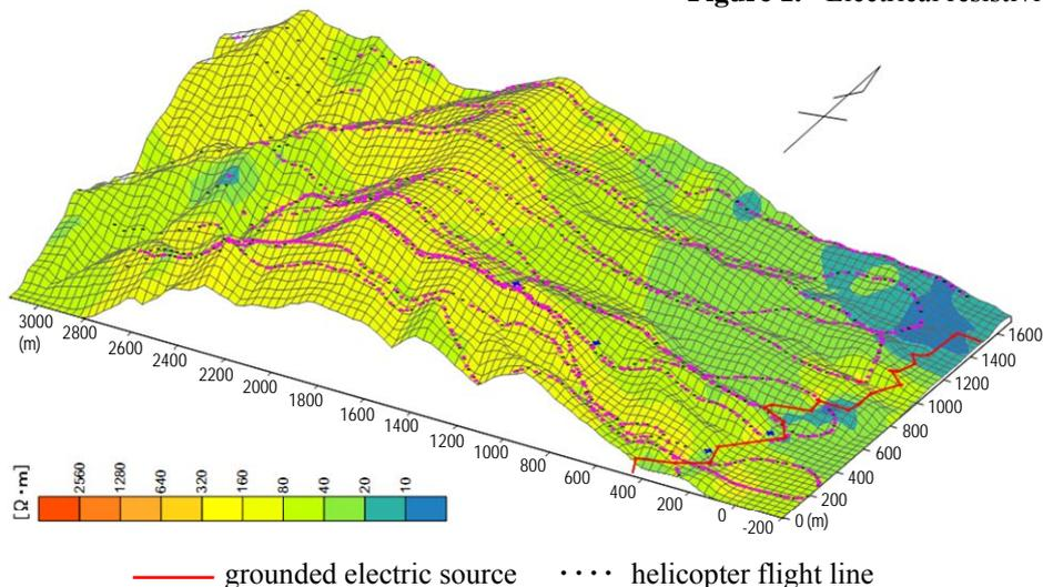
Figure 2. Electrical resistivity distribution of tunnel site surface.
