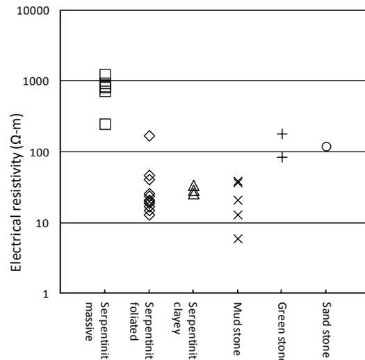
Figure 1. Electrical resistivity of rocks.
