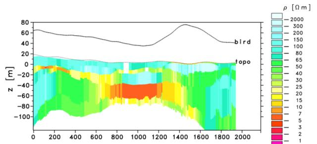
**Figure 3:** Vertical section assembled of 1D inversion results of real data. The location of the profile is indicated by a white line in Figure 2.
