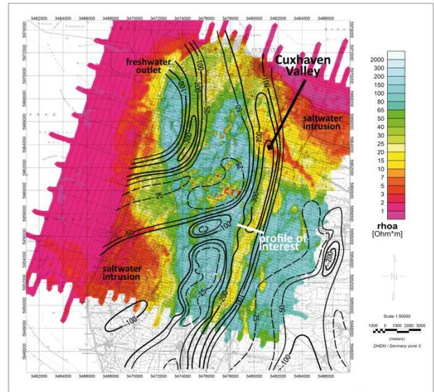
**Figure 2:** Apparent resistivity map derived from HEM data at a frequency of 1.8 kHz (after Siemon et al., 2001) including contour lines of the Quaternary base in meters (after Kuster and Meyer, 1995). The white line shows the location of the profile of interest.
