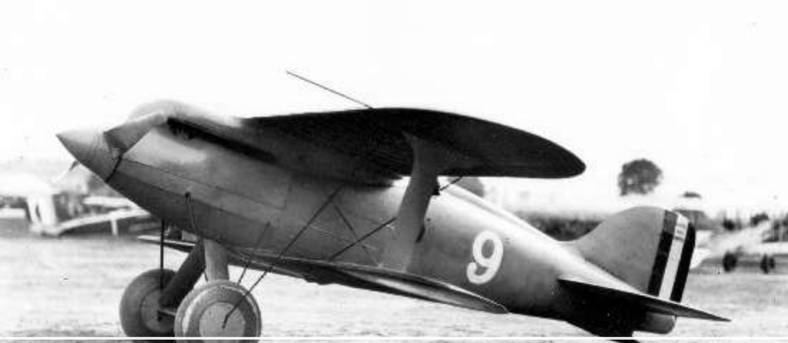
Curtiss R2C-1 Racer mid-1920's (248.97 mph). D-12 Engine 507 HP
