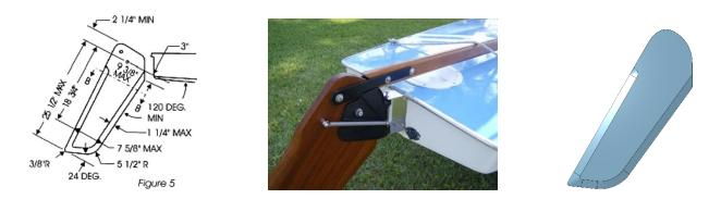
Left: Design of 2020 ISCA Class Legal Sunfish rudder. Center: The rudder attaches to the hull through a gudgeon bracket and spring-loaded pintle pin. Note the convenient pop-up feature which should be retained in a new design. Right: legacy rudder blade as modeled in Onshape CAD.
