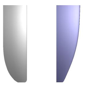
Left: Legacy daggerboard for the Sunfish. Right: New daggerboard using the design and fabrication procedures developed for the FS rudder blade. Water flow is from right to left in both cases. (only geometry below hull shown)
