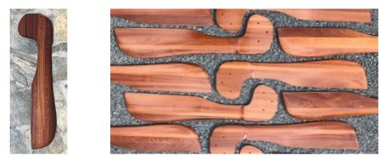
Above: first production FS rudder blades, provided with holes for quick replacement in the standard attachment hardware.
