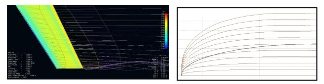
Left: CFD results for baseline/legacy rudder, showing pressure on the suction surface and flow streamlines. Right: Side force distribution for 0-10 degrees leeway, shown from the blade's lower tip (left) to the waterline (right), shows poor correlation with the optimal distribution, depicted by the gray curve for 5 degrees leeway.
