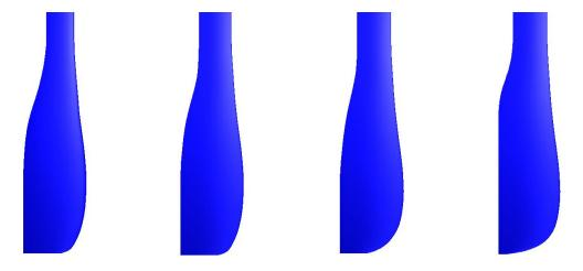
*Progression of rudder shapes during design iterations. Small, subtle changes resulted in an increase of the CL/CD ratio by 8% from the shape on the far left to the final design shown on the far right.*
