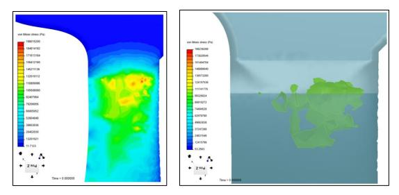
*Left: stress distribution (von Mises stress) on the surface of the FS rudder blade just below the waterline. As expected, the highest stresses occur at the thinnest parts of the blade. Right: isosurface (green) defining the region within the rudder blade where the predicted loads exceed the strength of sapele wood.*
