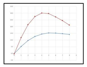
*CL/CD versus angle of leeway for the baseline legacy rudder blade (blue) compared to the new "FS" rudder blade (red).*
