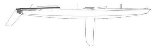
Sunfish hull and current Class-Legal rudder blade and daggerboard.
