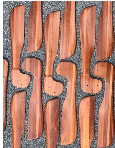
Following a year-long intensive development, AeroSouth this week has begun shipments of its revolutionary new rudder “FS” blades for Sunfish sailboats. The FS rudder blade promises a 50% reduction in drag and significantly lower weather helm compared to the legacy shape now used by recreational and competitive sailors on the world’s most popular sailboat.
