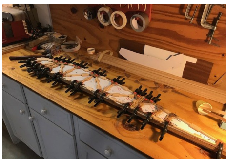
Above: rib #34 of 40, for the upper wing aileron sections. Right: rib jigs cut from thick shelf board.
