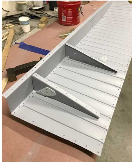
Very light coat of self-etching primer. Mar-Hyde in this case.
