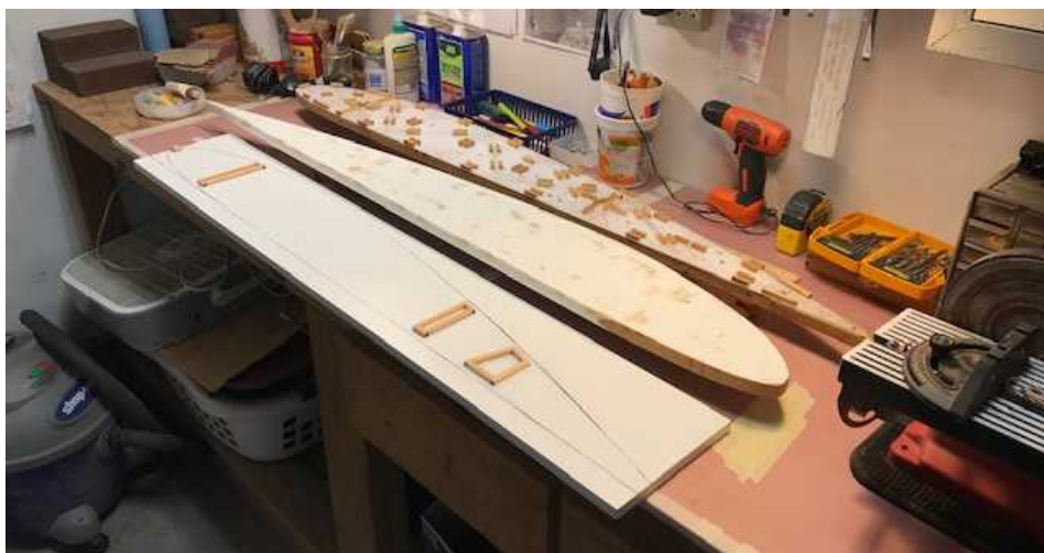
Above: std. rib jig, flat "back side" rib jig and spar jig (top to bottom).
