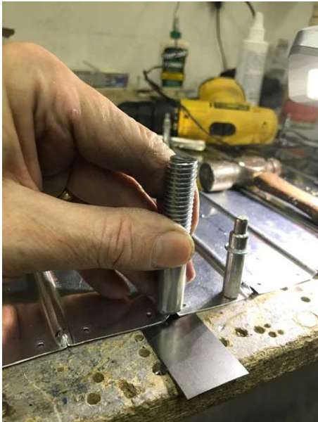
Technique is to tap the tool first vertically.
