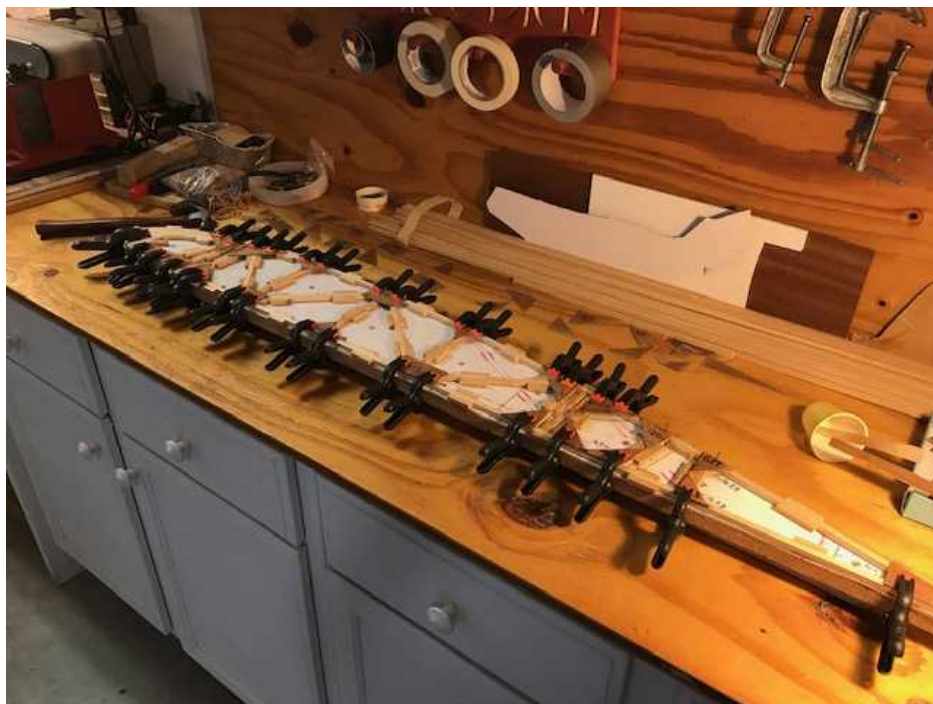
Above: Aileron rib during construction. Right: Completed ribs hung safely out of the way.
