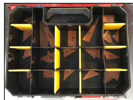
A plastic box with partitions for small parts made an ideal means of storing gussets while making the ribs.
