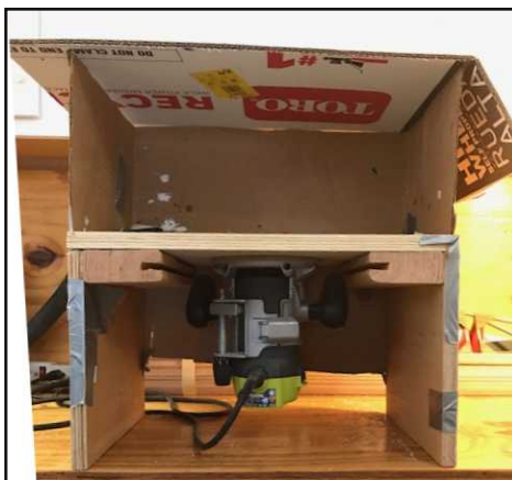
Above: Simple tabletop router made from a hand router and some wood scraps. The end of a Shop Vac hose was inserted in the top and held near the router bit. Below: router template and several of the nose pieces prior to finish sanding.
