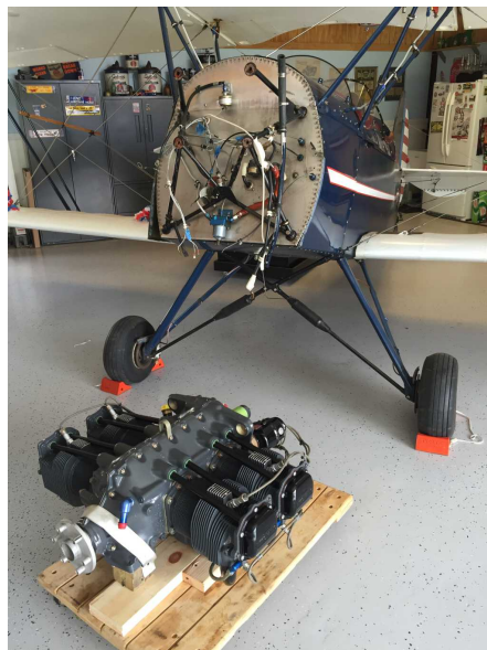
Left: rebuilt O-290 ready to go back on. Above: engine builder Joe Erale (right) and I discussing how we will recover the center section. Below: first engine run in seven years.
