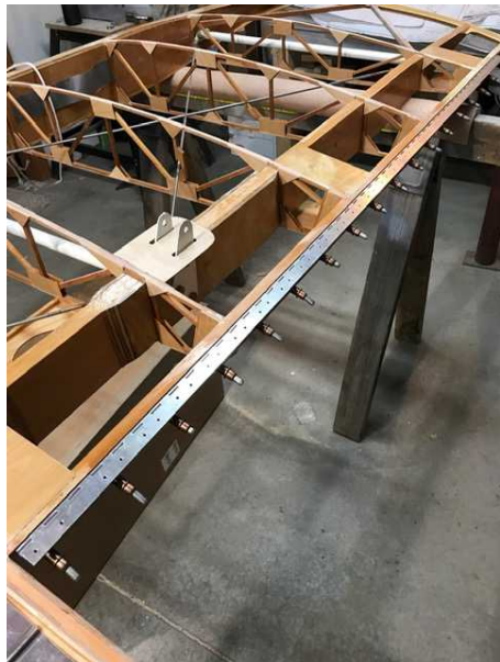
Hinge drilled to the wing prior to riveting. T-nuts retain the screws, and the flanges of the T-nuts are encased in micro fill thickened epoxy to prevent pushing them out on final assembly.
