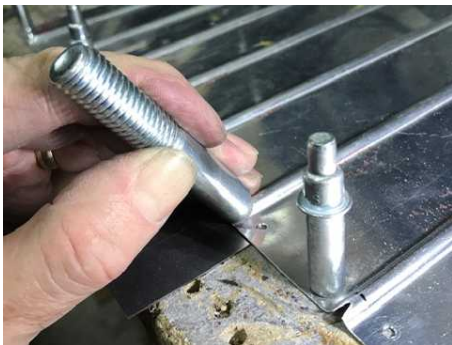
Then continuing to tap, roll the tool toward the edge of the skin. I have a piece of .025 steel at the edge of the sheet/corrugations to aid closing the corrugations.
