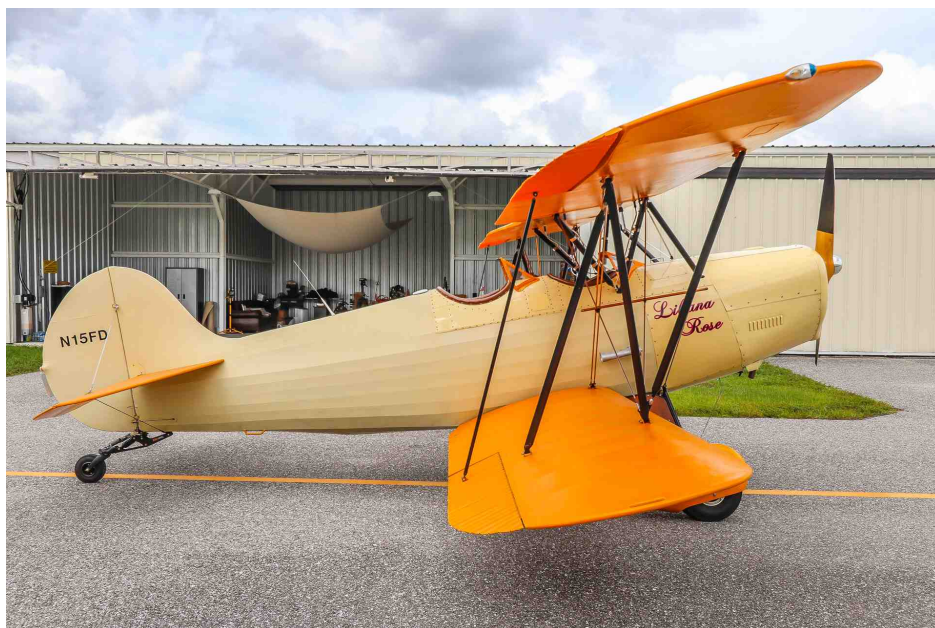
Bill went with the Alaskan Bush-Wheels T-3 tailwheel suspension with ABI-3224A tailwheel.
