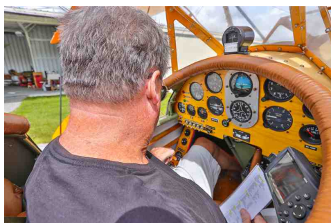
Bill adjusted the dimensions slightly to better handle the build of a firefighter: "The upper longerons are 3" higher than on the plan. Also, the cockpit is 2" wider to accommodate my shoulders." The panel includes ADS-B out, an ICOM A-210 radio, and a Garmin 396.
