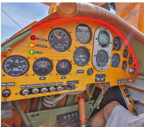
Bill adjusted the dimensions slightly to better handle the build of a firefighter: "The upper longerons are 3" higher than on the plan. Also, the cockpit is 2" wider to accommodate my shoulders." The panel includes ADS-B out, an ICOM A-210 radio, and a Garmin 396.
