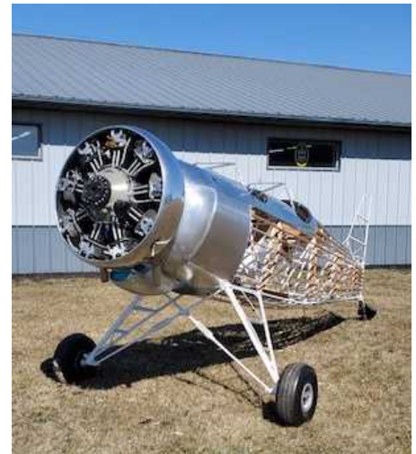
A bunch of speed ring brackets made. I used one on each head (9). Less may be possible, personal choice.
