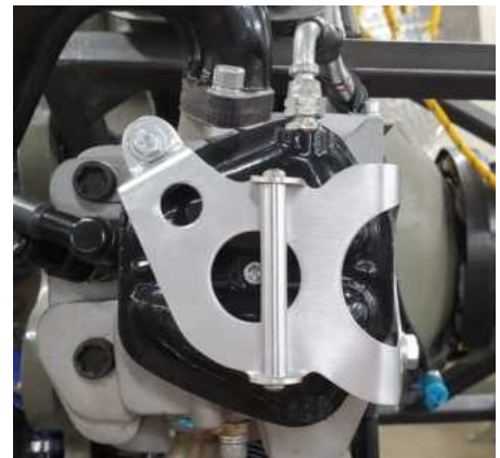
Top view of a speed ring mount bracket .
