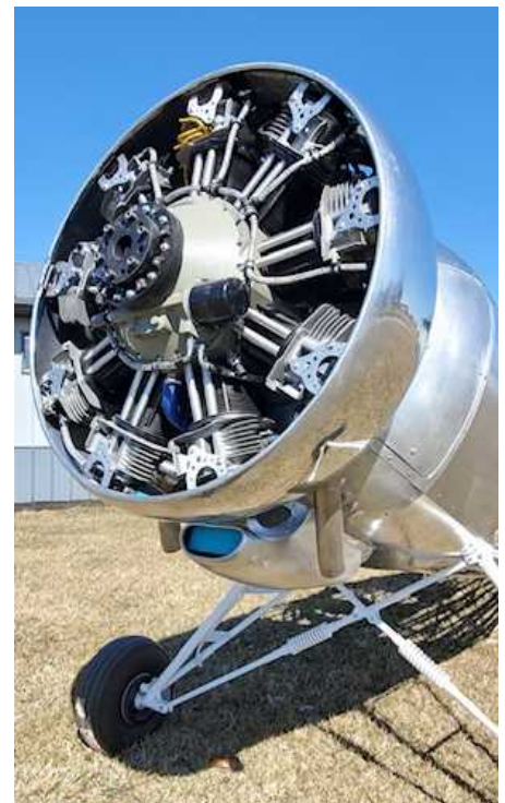
Right: Speed ring, dishpan and other aluminum skins attached. "OMG" is all one can say [editor]
