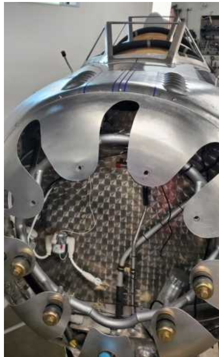
Close in dishpan shot. You can see the air/oil separator line running down, some wiring and engine turned firewall.
