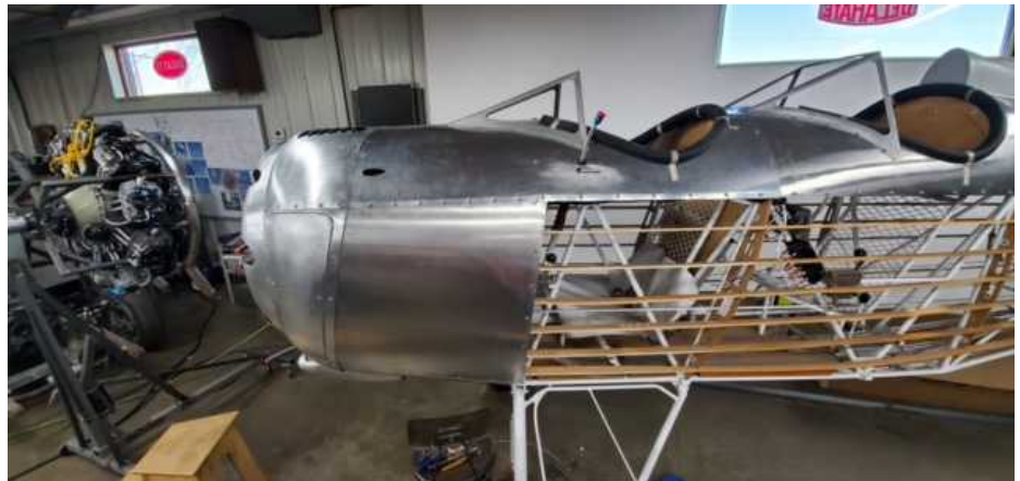
Moving engine close on a stand to check fits and clearances.
