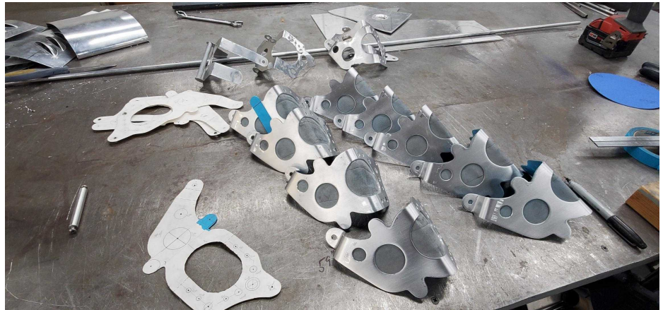
A bunch of speed ring brackets made. I used one on each head (9). Less may be possible, personal choice.
