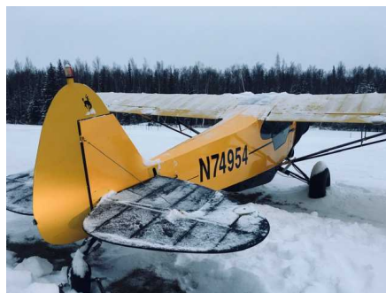
The black fabric here is Oratex, the fuselage from Stewart's and the wings are Superflite poly.
