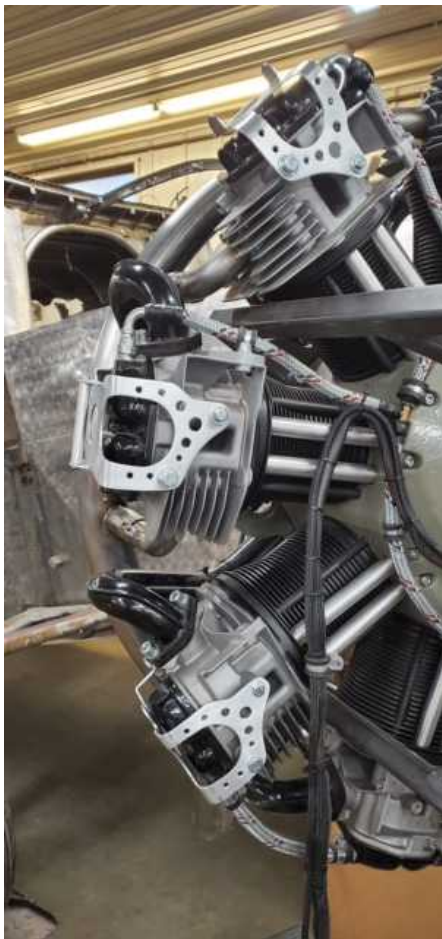
Side view of speed ring brackets.
