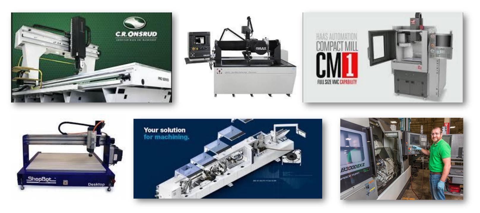
**Computer Numerical Control (CNC)** - the automated control of machining tools and 3D printers by means of a computer. A CNC machine processes a piece of material to meet specifications by following a coded programmed instruction and without a manual operator directly controlling the machining operation. G-code and M-code commands provide instructions to CNC machinery.
