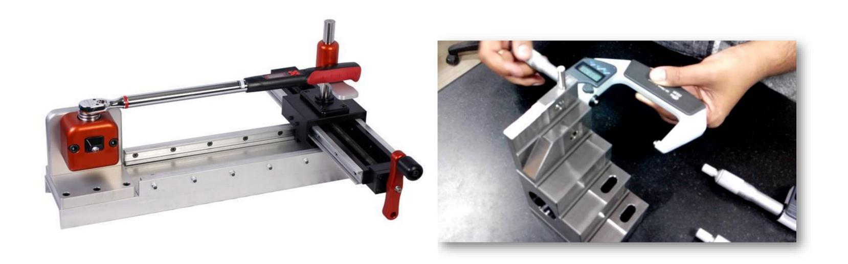
Regular **calibration** assures that an instrument shows results that are **accurate**, ie they match accepted values, within **allowable tolerances**. In industry, **regular calibration** by experts may be required by **contract or law**. Above: calibration of a torque wrench and a micrometer.
