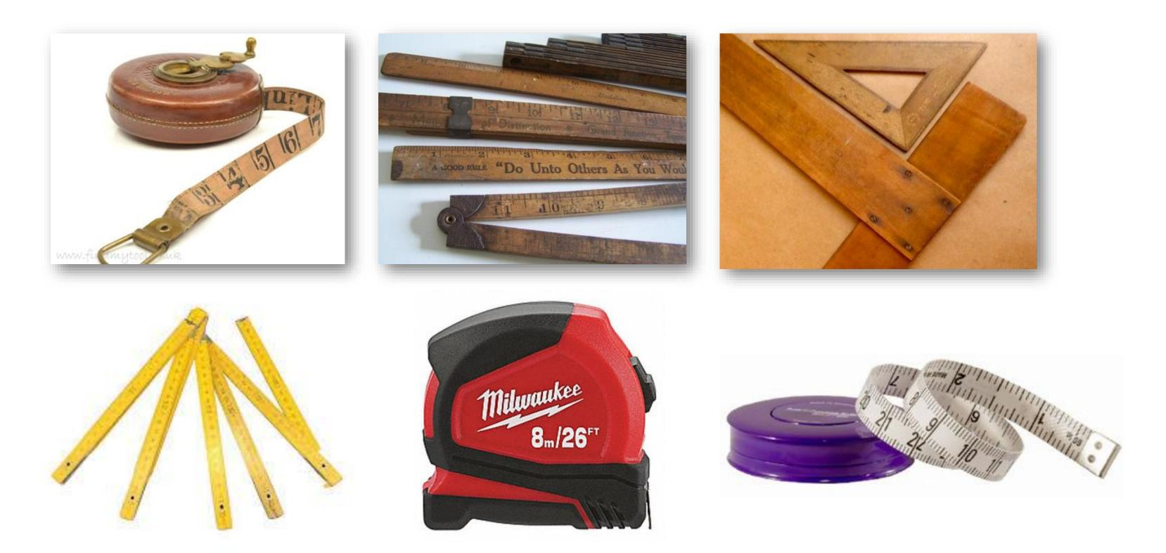
Flexible (tailor's) measuring tape, old wooden rulers, folding ruler, tape measure, old wooden T-square and triangles. Temperature and humidity fluctuations change wood's dimensions. Wood is also easily damaged.
