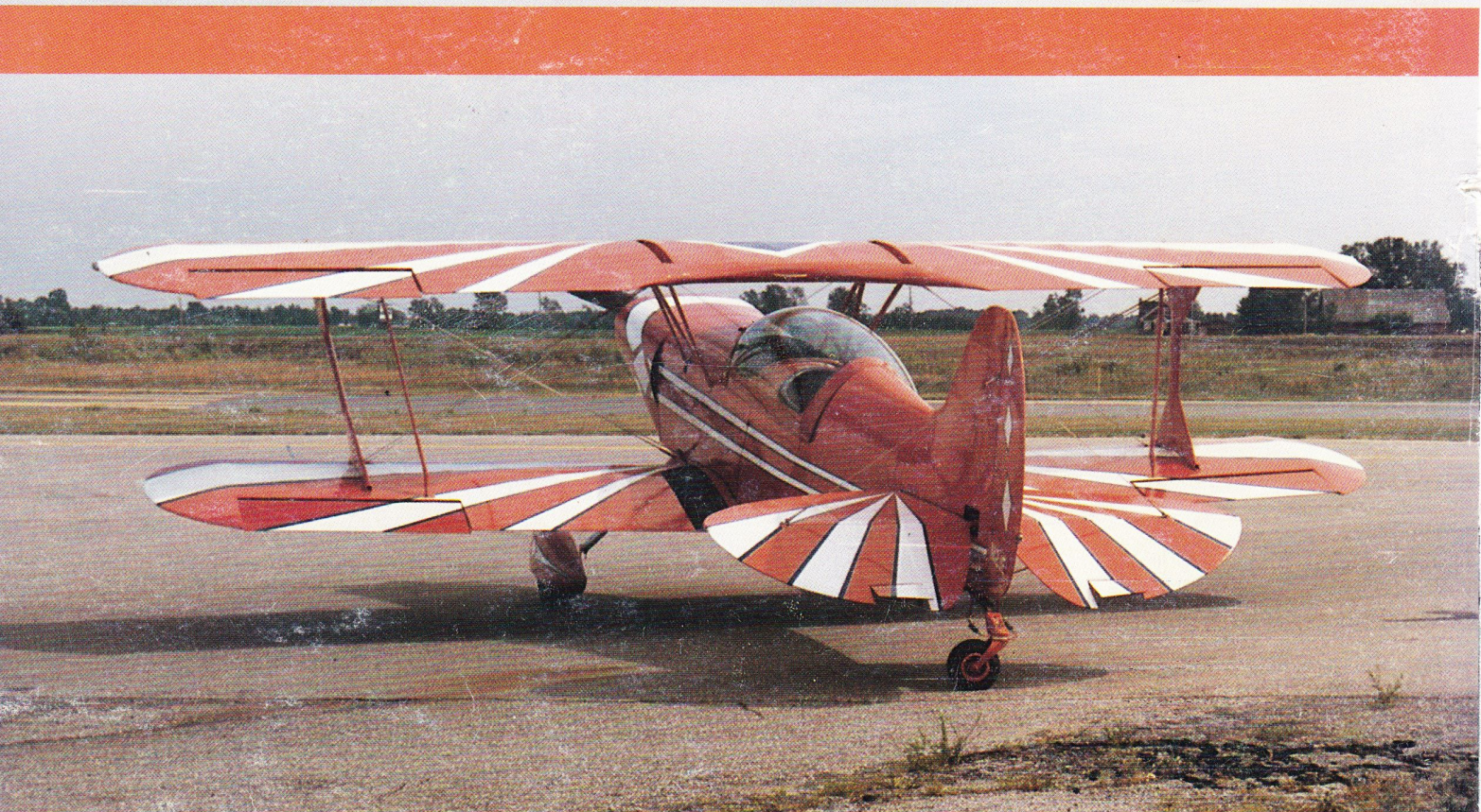
Jack Elenbaas, Holland, MI installed a one-piece canopy on his Acro II for year-round flying. Aircraft also modified with a spring steel gear. Engine is a 165 hp 4-cylinder Continental IO346A.
