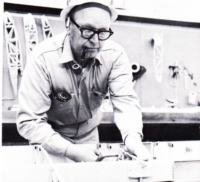
Positioning wing ribs on the wing spars. Rib positions are accurately measured and penciled on front and rear spars before sliding ribs into position.
