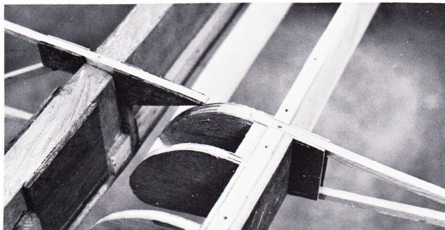
Acro Sport ailerons prior to trailing edge being installed. All wood internal parts should be varnished prior to covering.
