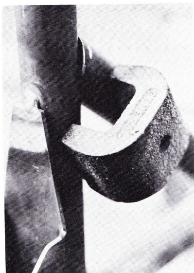
Magnet used to hold tubing into position while tack welding.
