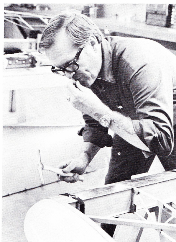
Bob Ladd nails pre-formed leading edge in position. Note adjustable straps that hold aluminum leading edge tightly in position.
