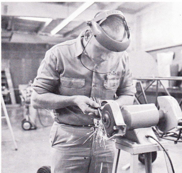
Always wear safety shield or safety glasses when grinding metal fittings.
