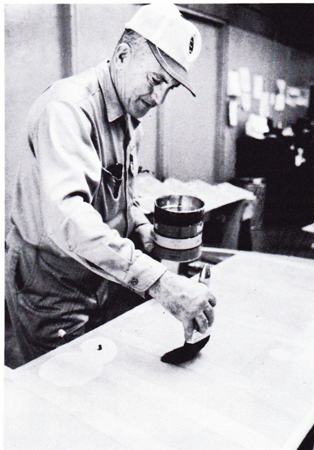
Smooth, easy strokes are used in applying dope. Keep dope from thickening by adding a bit of thinner.
