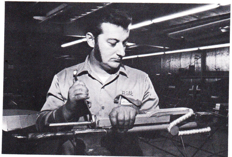
Putting shock cord in place with landing gear shock strut.
