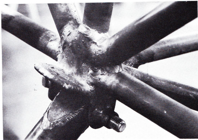
Front landing gear and double flying wires fitting offers sturdiness.
