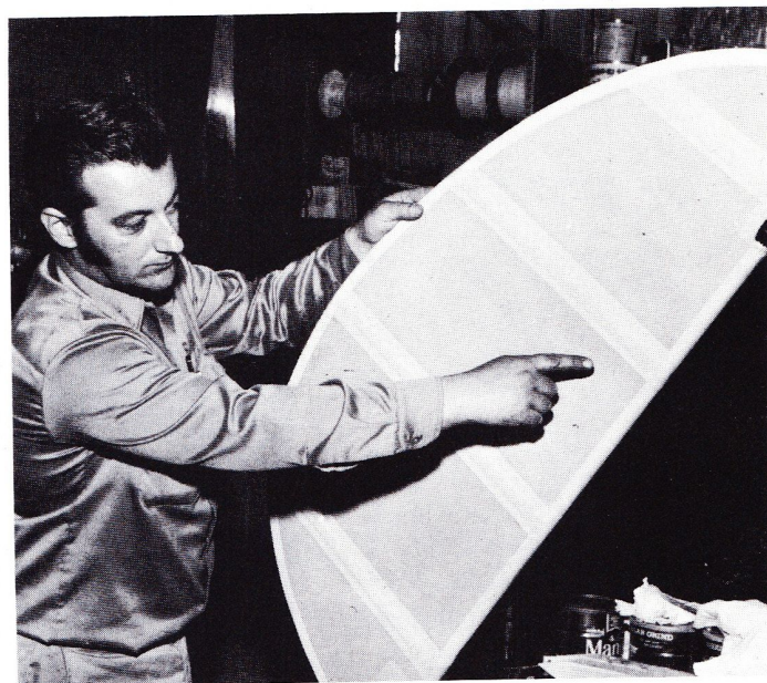
Pinked tape is used to cover ribs and leading and trailing edges.
