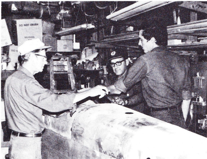
Here is a fuselage assembly taking place in a one car garage shop. On completion components such as wings are often suspended from overhead rafters.
