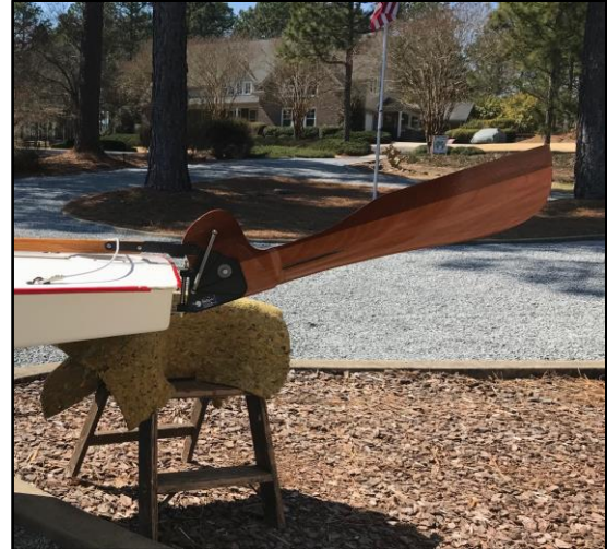
Left: Rudder in upward position when tiller strap is attached to the “standard” hole in the head of the blade. Right: Rudder in upward position when tiller strap is attached to the “modified” hole in the head of the blade.
