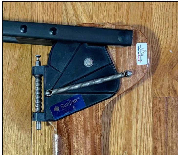
Sunfish cheek flange combined with wishbone-style tiller. Note special location of hole for the tiller in the drawings on page 2. (Image courtesy Sunfish owner Rick Schlosser)
