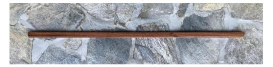
**Purpose:** Steering lever attached to the head of the rudder.
