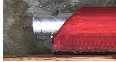
*Left: Tube sleeve and three supplied 1/8" x 1" SS pan-head screws. Soft foam adhesive strip is used to help position sleeve and account for non-planar surfaces. DO NOT OVER-TORQUE SCREWS WHEN ATTACHING OR PLASTIC MAY BREAK! Right: Supplied cotter pin installed through hole at the end of the aluminum tube.*
