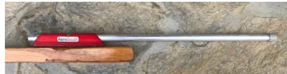
*Left: Tiller extension fully retracted, limited by plastic cap, which is bonded to the end of the tube. Sleeve is attached so that the end of the aluminum tube is somewhat behind the end of the tiller when retracted, eg 1"-2". Right: Tiller extension fully extended, limited by cotter pin.*
