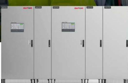
Gutor PEW is an industrial online double conversion single-phase UPS system with thyristor-controlled rectifier and IGBT-PWM inverter designed to secure critical applications in harsh environment.
