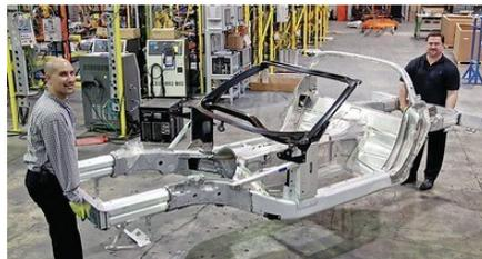
weight race was in full swing. In 2001 the titanium exhaust system of the Z06 weighed a mere 26lbs, a 70% reduction from the conventional exhaust! A new aluminum alloy frame reduced the frame weight by nearly 20%, a saving of over 100lbs, yet increased body rigidity!
