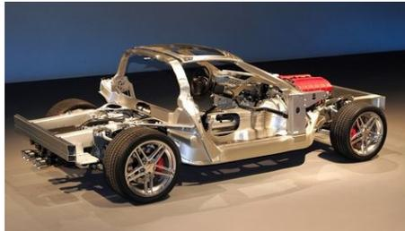
Additionally GM began messing around with unique frame materials, such as titanium and balsa wood (yes your C5 & C6 Corvette has balsa wood in the floor boards) to further reduce the overall weight of the car. GM was chasing weight reduction everywhere, the new motor in the C5 was 10lbs lighter than that of the C4 yet still increased the Horsepower!
