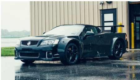
2011 mid -engine Mule that was used to develop the C8 design
