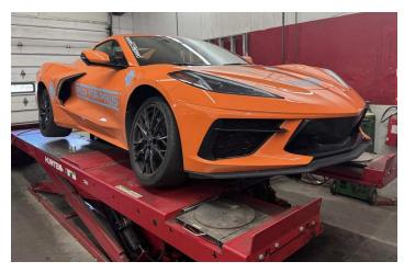
properly placed, the car will fall of the lift as it goes higher in the air! Gravity always wins!
