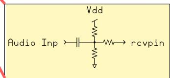
All resistors: 2.2 K $\Omega$ All capacitors: 0.1  $\mu$ F
