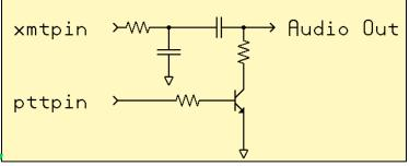
All resistors: 2.2 K $\Omega$ All capacitors: 0.1  $\mu$ F Transistor: 2N3904
