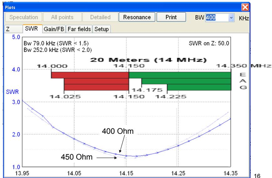
Just to make sure that 450 Ohm cable is not going to disrupt totally the ZS6BKW run with 400 ohm transmission line proposed by Brian Austin, here are both plotted together. They are very similar and that is true for most of the bands studied.
