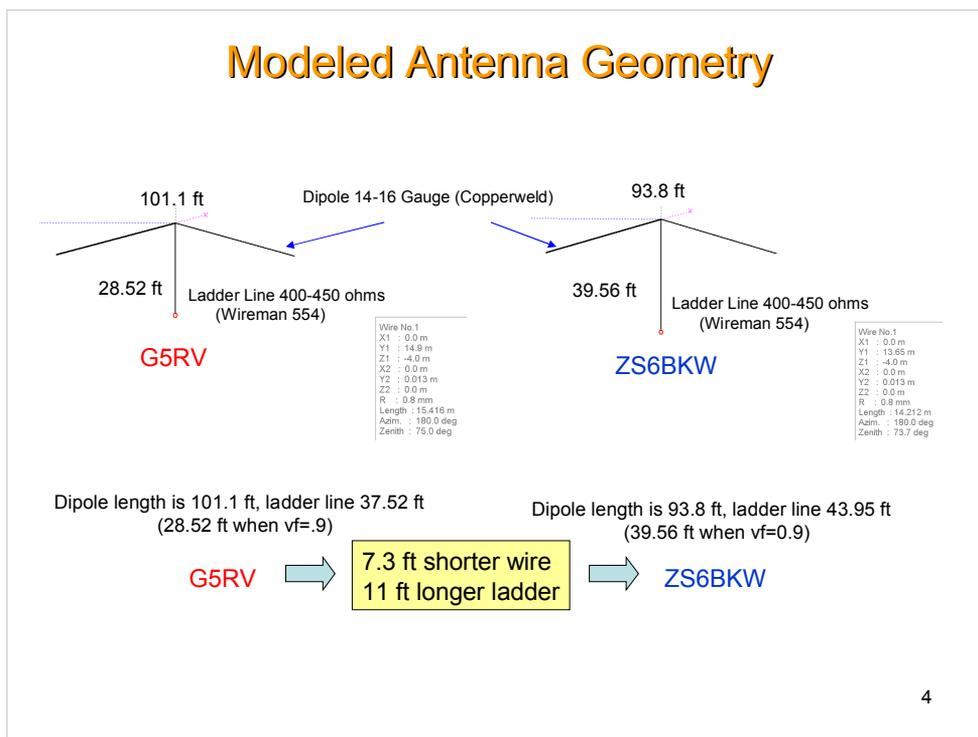
The design of both antennas consist of a dipole configuration fed with a length of ladder line. I use copper coated steel for the dipole portion because I use the antenna wire as a partial support for the insulated pole supporting the antenna.
