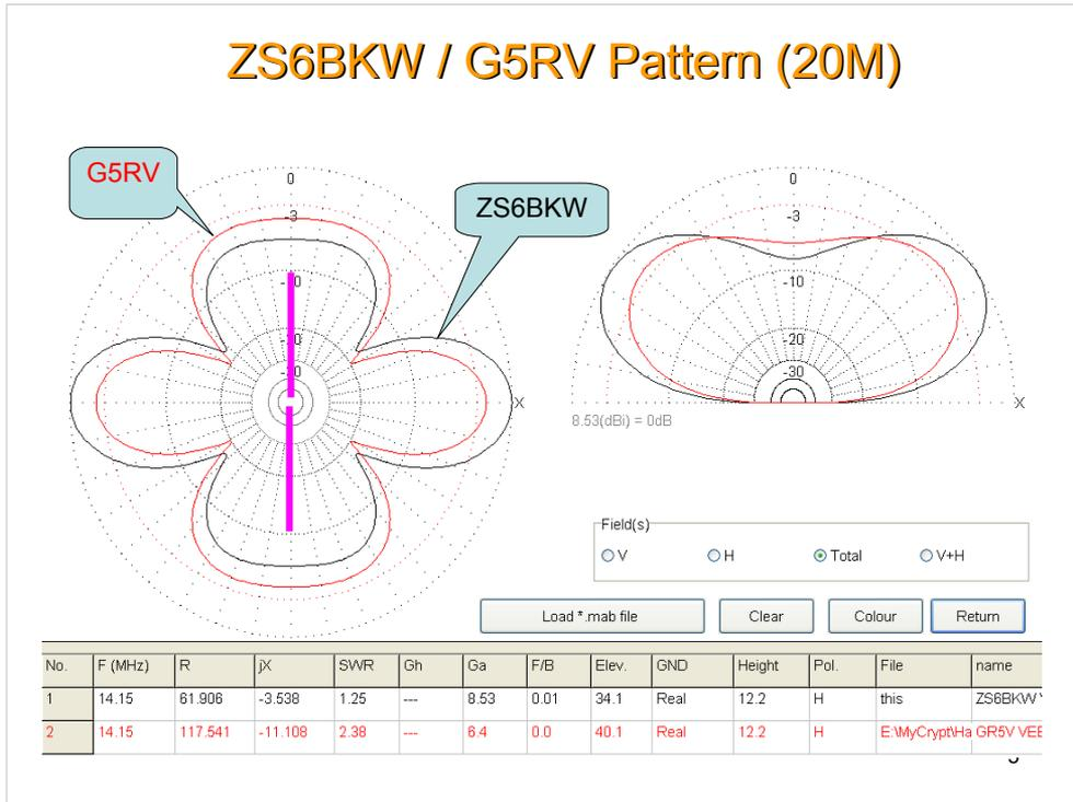
The antenna patterns are very similar because the radiating antenna lengths are fairly close. This is true for each band analyzed. The ZS6BKW being shorter exhibits less pattern variation because it is closer to a standard dipole on most bands.
