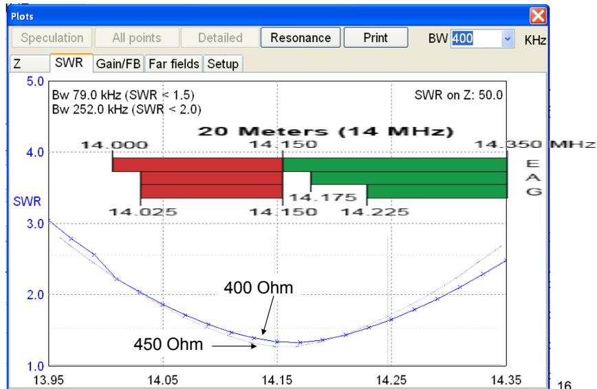
Just to make sure that 450 Ohm cable is not going to disrupt totally the ZS6BKW run with 400 ohm transmission line proposed by Brian Austin, here are both plotted together. They are very similar and that is true for most of the bands studied.
