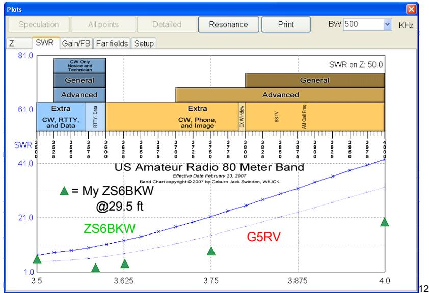
This indicates that the G5RV is **marginally** better than the ZS6BKW on the 80 meter band. However, both exhibit unsatisfactory SWR and would require a tuner to match it to your transmitter.
