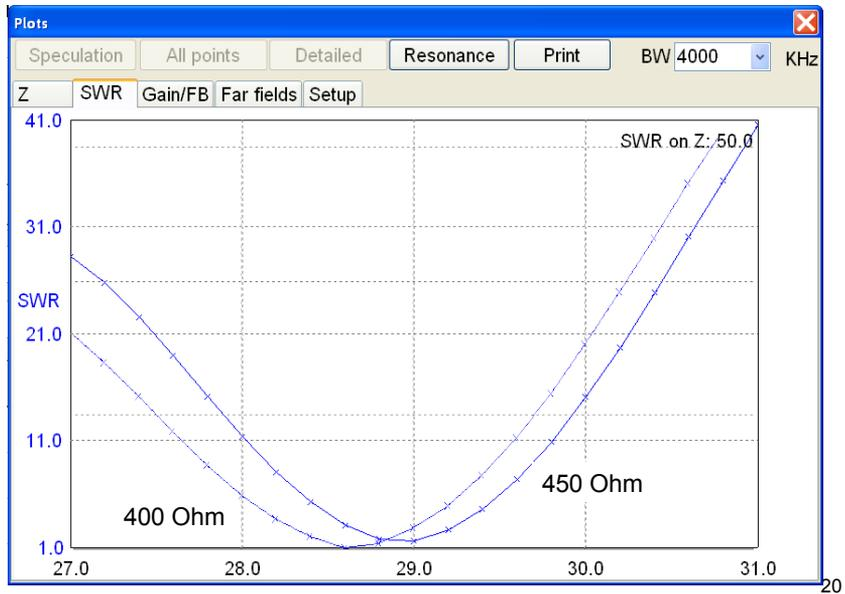
The frequency of minimum SWR is shifted a little lower, but the useful range of the antenna is still limited.
