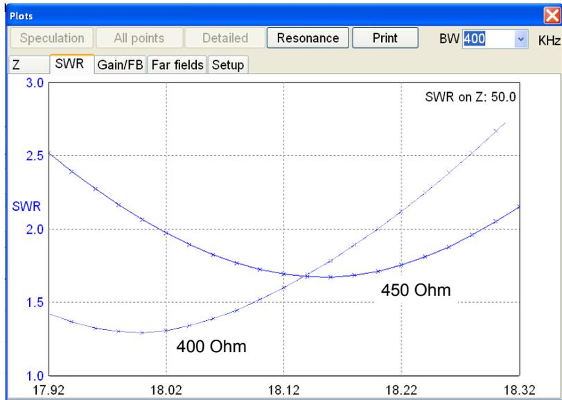
This band is not helped much by using 400 ohm line, although there is a difference in SWR curves.
