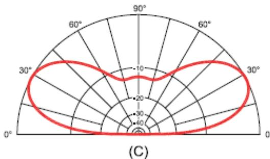
Antenna height changes the resulting antenna pattern, starting with mainly high angle radiation at 1/8 wavelength then progressing through a lowering of the high angle radiation as one approaches 1/2 wavelength. Then it grows more high angle radiation and then breaks into “lobes” at distinct take off angles. Note that 1/2 wavelength on 20 M is about 33 ft (C). This would give the antenna good DX on that band since the energy would not all be “used up” radiating straight up.
