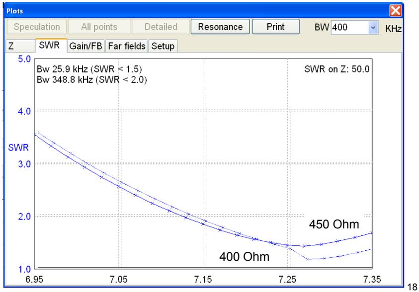
The 40 meter band is not significantly different with either line feed.
