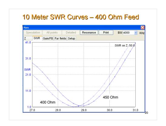
The frequency of minimum SWR is shifted a little lower, but the useful range of the antenna is still limited.
