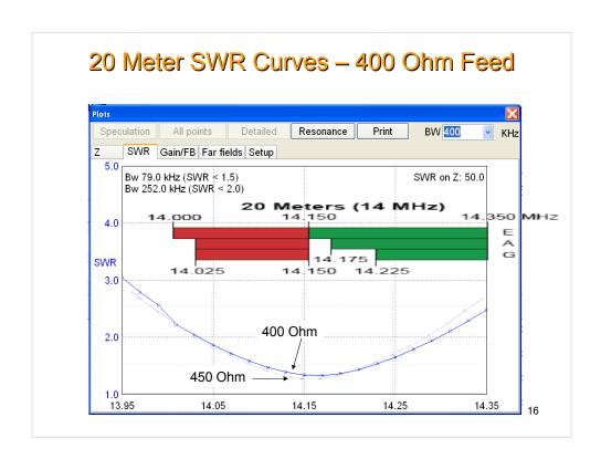
Just to make sure that 450 Ohm cable is not going to disrupt totally the ZS6BKW run with 400 ohm transmission line proposed by Brian Austin, here are both plotted together. They are very similar and that is true for most of the bands studied.
