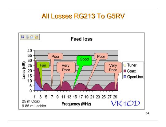
The above data is taken from the VK1OD web site. He has performed extensive computer analysis using NEC modeling software and custom computations, computing total system losses for the G5RV antenna with different feed systems. The data is not available for the ZS6BKW, but because the SWR is lower within the same ham bands, the losses will be lower as well.
