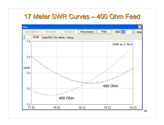
This band is not helped much by using 400 ohm line, although there is a difference in SWR curves.
