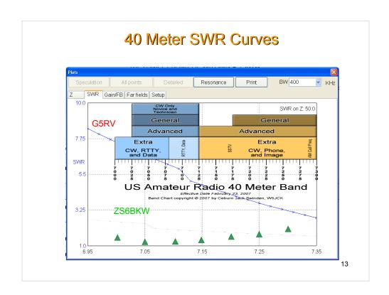
The 40 meter band is a natural for the ZS6BKW antenna. Its length is longer than a half wave and thus has some gain over a dipole in the broadside direction.
