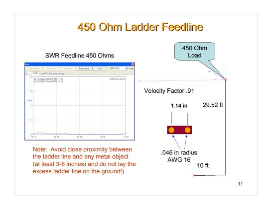
The slide shows the parameters used to model the feed line for both the G5RV and the ZS6BKW antennas. A resistive load was applied at the apex of the antenna instead of connecting the antenna wires. The SWR graph indicates that the model is realistic, at least when the load is matched to the line.
