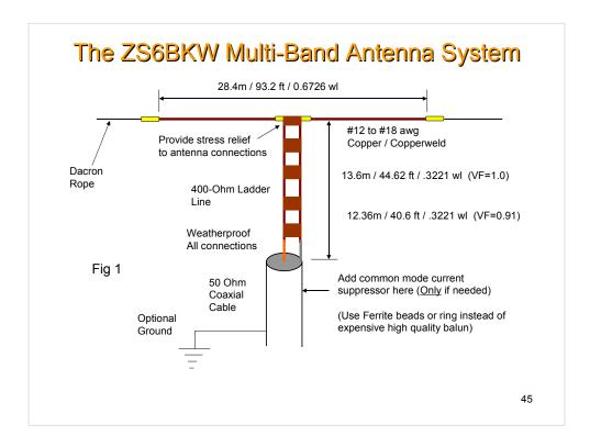
The above is the flat-top version of the ZS6BKW antenna. Note especially the location for torroid suppressor choke (only if required.) Do not assume that you will need a choke. Another choke is to wind about 10 turns of your coax run on a form of about 6 incles.
