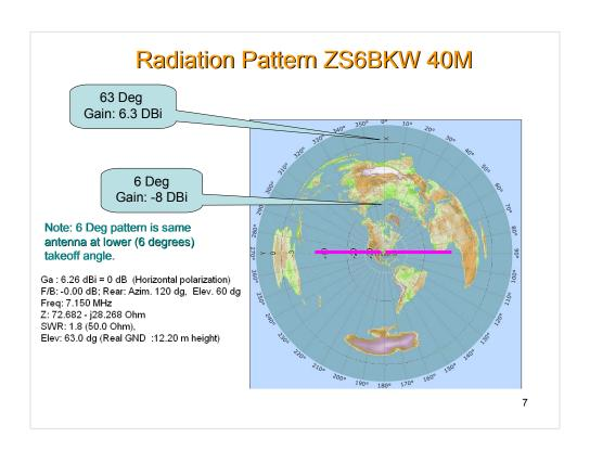
Forty meters has a slight directive pattern broadside to the antenna. It has some gain over a 40 M dipole at the same height.
