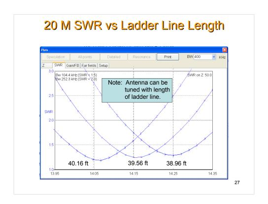
The ladder line is the "magic" that allows the ZS6BKW to match so many bands. Here we see that we can change the resonant point in the 20 meter band simply by adjusting the ladder line length. However, the characteristics of the other bands will change as well. If you have a favorite portion of a band, more than likely the antenna can be optimized for that portion of the band.
