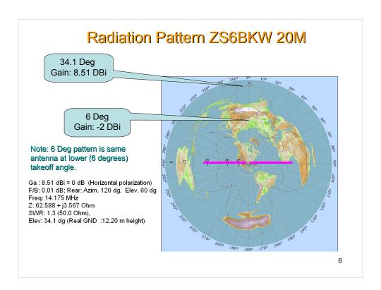
These plots are overlaid on a great circle view of the world to be able to visualize the preferred directional coverage of the antenna. I arbitrarily chose to orient the antenna broadside North to South for visualization. In my own installation, I have the antenna broadside and a little to the West of due north because of my choice of supports.
