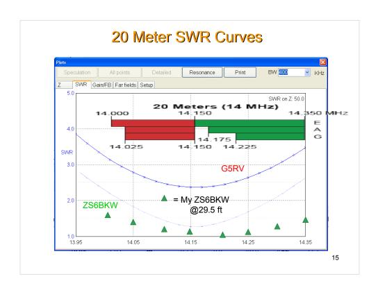
This is the band that the G5RV was specifically designed to cover with both low SWR and a usable pattern. The ZS6BKW will have slightly lower losses and will match the transmitter over a larger portion of the band. However, both antennas should perform well on this band. The orientation of the antenna can make a significant difference in what areas are covered by the antenna pattern.
