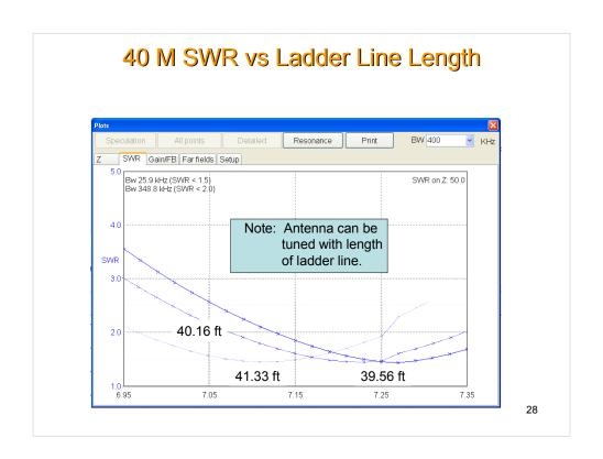
The frequency can also be shifted in the 40 meter band. It can be "tuned" for either the CW portion or the phone portion of the band.
