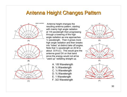
The pattern change on either antenna with height is minimal for practical amateur installations. The effects are more noticeable at the higher frequencies.
