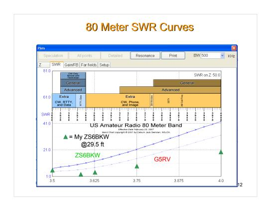
This indicates that the G5RV is marginally better than the ZS6BKW on the 80 meter band. However, both exhibit unsatisfactory SWR and would require a tuner to match it to your transmitter.
