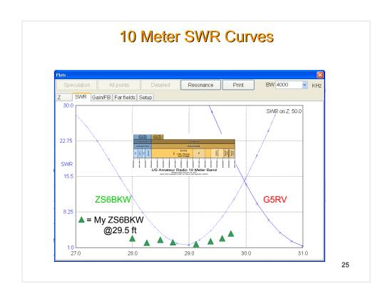
The ZS6BKW resonates in the 10 meter band. However, it will not cover the entire band without a tuner. The G5RV resonates outside the band. It will not perform well on 10 meters with high losses due to the SWR. Note that the measured SWR is MUCH better than the modeled antenna SWR. This is because of the losses in the cable run to the antena at this frequency.
