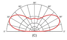
Antenna height changes the resulting antenna pattern, starting with mainly high angle radiation at 1/8 wavelength then progressing through a lowering of the high angle radiation as one approaches ½ wavelength. Then it grows more high angle radiation and then breaks into "lobes" at distinct take off angles. Note that ½ wavelength on 20 M is about 33 ft (C). This would give the antenna good DX on that band since the energy would not all be "used up" radiating straight up.
