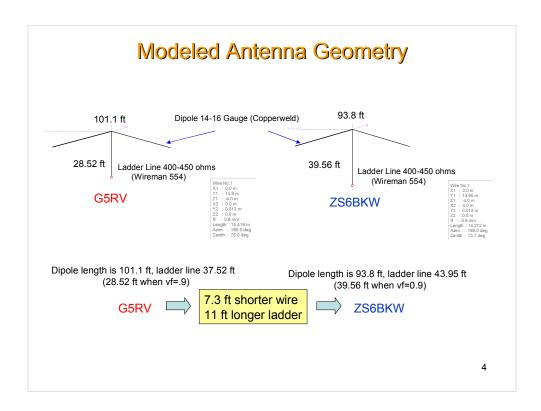
The design of both antennas consist of a dipole configuration fed with a length of ladder line. I use copper coated steel for the dipole portion because I use the antenna wire as a partial support for the insulated pole supporting the antenna.
