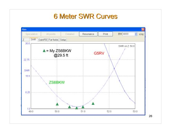
Interesting that it also resonates within the 6 meter band. The G5RV would have high losses over the entire band.
