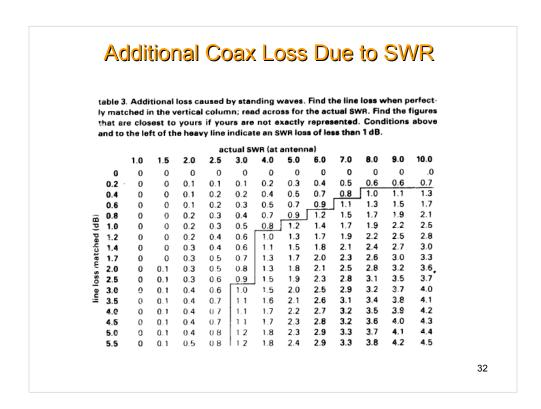
This chart tells the story behind the concern expressed in this presentation. If you have losses in your coax (and you will have loss) and if the SWR at the load end of the coax is high, you will have lost some (or most) of the power you put into the coax at the transmitter end. This is even before it gets a chance to radiate.
