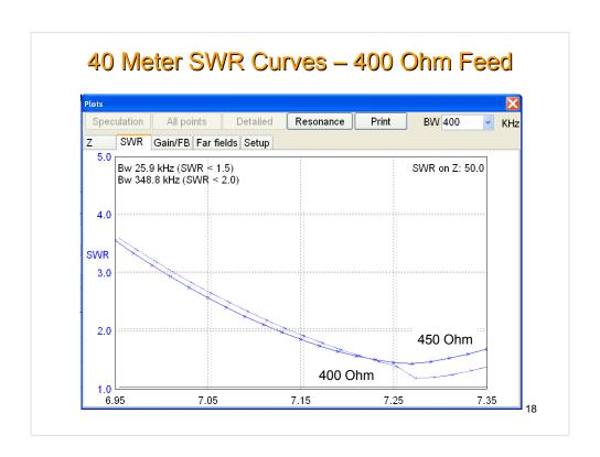
The 40 meter band is not significantly different with either line feed.
