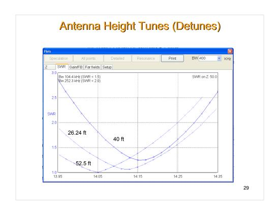
There is a small dependence of the SWR with height. This is true for all antennas and not unique to the ZS6BKW and G5RV. It is also true for the standard dipole. This can be factored into your modeled design of the antenna for optimum results.
