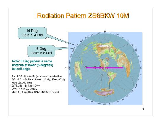
The antenna pattern on 10 meters has considerable gain with multiple lobes. It also has good low angle radiation, even at the modest height of 12.2 meters.
