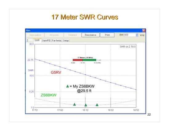
The 17 meter band is one of my favorite bands. It looks like it matches fairly well over the majority of the band. The G5RV will not match well, and when matched by a tuner will have significant losses. (> 3 DB loss or half the power.)
