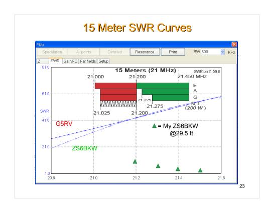
Both antennas are poor on this band. I do not understand why I measure fairly good SWR on this band. Most likely my particular length of coax is acting as an impedance transfromer "matching" the antenna to the transmitter. I have not operated on this band and so do not know how well the antenna performs on this band.
