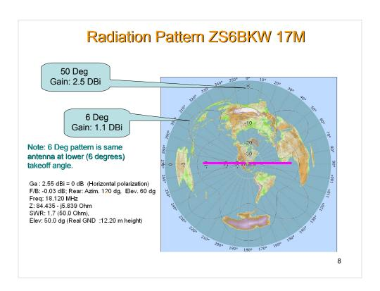
The antenna pattern changes with the elevation angle, so orienting the antenna may entail a tradeoff between stateside and DX coverage. Note the large pattern change at 6 degrees vs that at 50 degrees.
