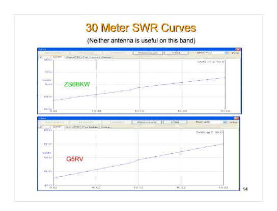
Neither antenna will provide satisfactory results on this band. The high SWR and the accompanying losses will make it difficult to make contacts on this band.
