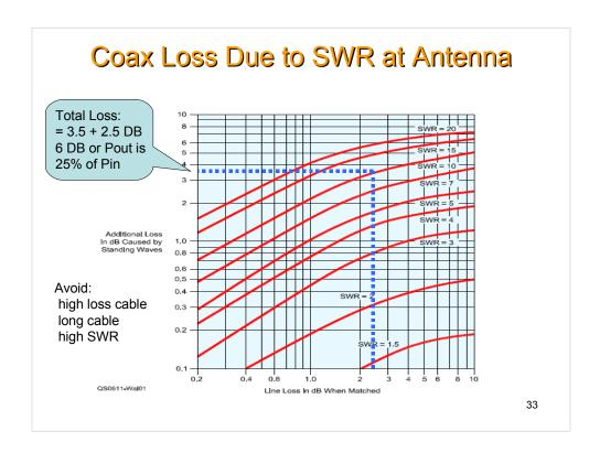
This graph shows that the losses in an ANTENNA SYSTEM is dependent on the cable losses as given by the manufacturer PLUS an additional loss due to the SWR of the load to which the coax is connected.
