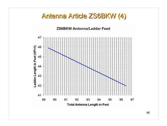
If you want to use different lengths for the ladder line or antenna, the above graph was provided by Brian Austin as part of his computer modeling. I have truncated the graph to a straight line through the center of his area graph for simplicity.
