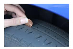
Thin tire treads create hazardous driving conditions when water builds up on the roadway, according to the Car Care Council. Deep tread accommodates accumulated water; thin tread does not. Thin tread causes the tire to hydroplane – ride up on a film of water, losing contact with the pavement, similar to driving on ice.
