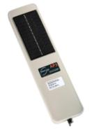
The AssetPack-3 (AP3) is a battery powered, solar-rechargeable tracker that can communicate with a full range of asset data. By listening to the asset communication bus via RS-485, MODBUS, CANBUS/J1939 or serial interface, AP3 provides unparalleled monitoring for assets that are off the grid. The additional ability to communicate with the device
