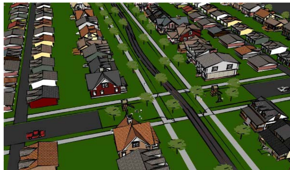
Figure 8 – Rendering showing how a full greenway treatment would replace a roadway with green space and a two-way bikeway, with sidewalks remaining. Alleyway access is not shown but would remain behind the houses fronting the greenway. Image courtesy of Transit for Livable Communities and Community Design Group.
