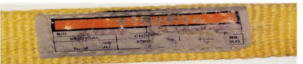
• Illegible or Missing Tag
