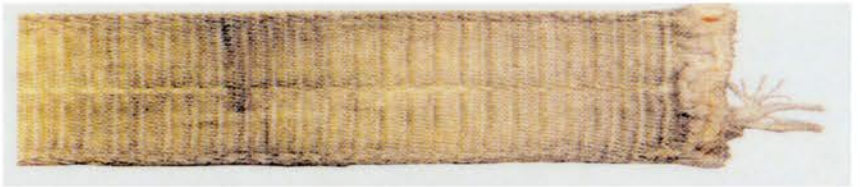
• Cut & Tensile Damage
