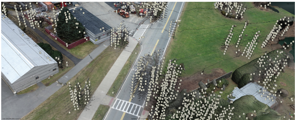
Figure 5. Measuring tree height using contour generation in Agisoft Metashape.
