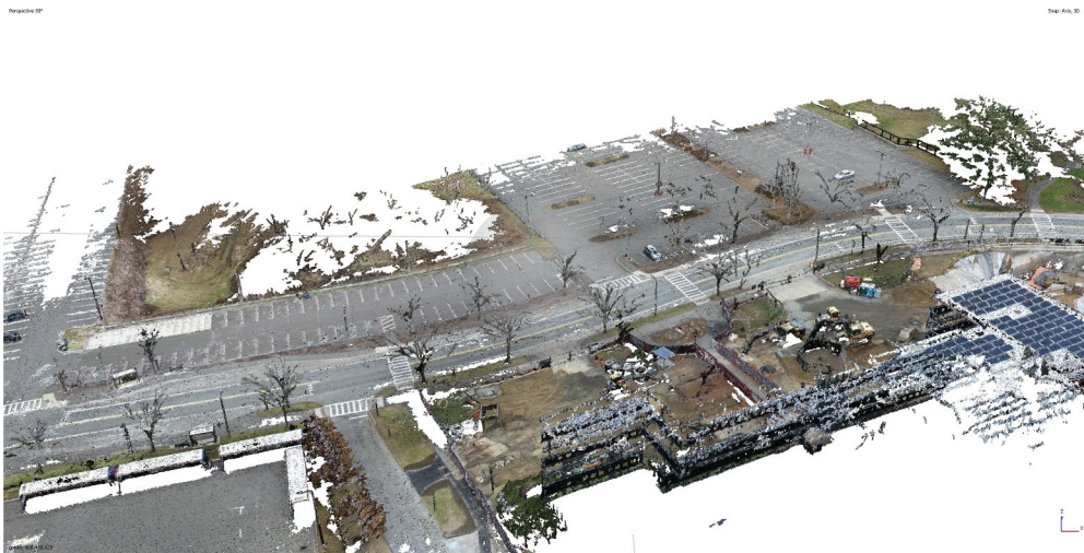
Figure 3. Structure-from-motion 3D model using leaf-off imagery in Agisoft Metashape. Governor's Drive, Amherst, Massachusetts.
