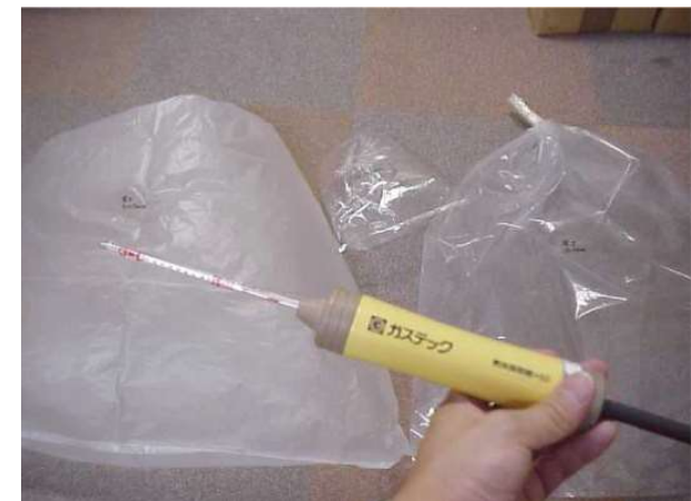
Compare the formaldehyde gas level between blank and test piece.
