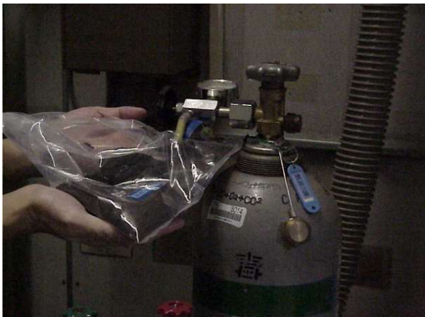
Formaldehyde gas is injected into the bag containing the test piece and the bag not containing the test piece.
