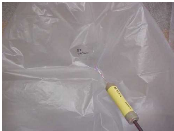
Measurement the gas level by the detection tube after placing those bags at optional time.
