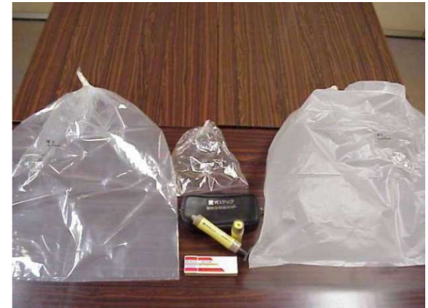
Tools : Gas detection tube, inspirator, plastic bags, formaldehyde gas
