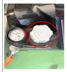
Adjust the air pressure level by the air pressure regulator valve.
