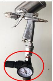
Adjust the air pressure level with an attachable air pressure regulator valve.
