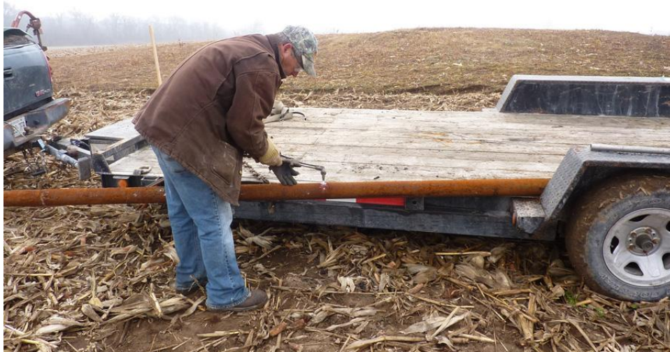
13 November 2010. Ken Young using a cutting torch to sever gas well pipe into sections suitable for the 6 corner posts marking the perimeter of the Cemetery.
