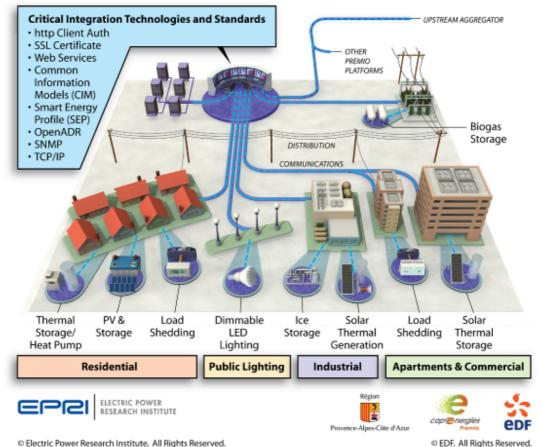
Figure 2 EDF EPRI Smart Grid Demonstration Host site
