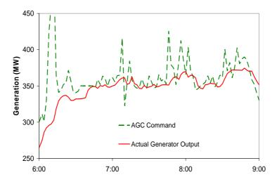
Figure 4 Conventional turbine generators sometimes follow AGC commands poorly.
