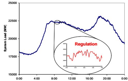
**Figure 8 Regulation Is the Response to the Minute by Minute Fluctuation in Net Load**
