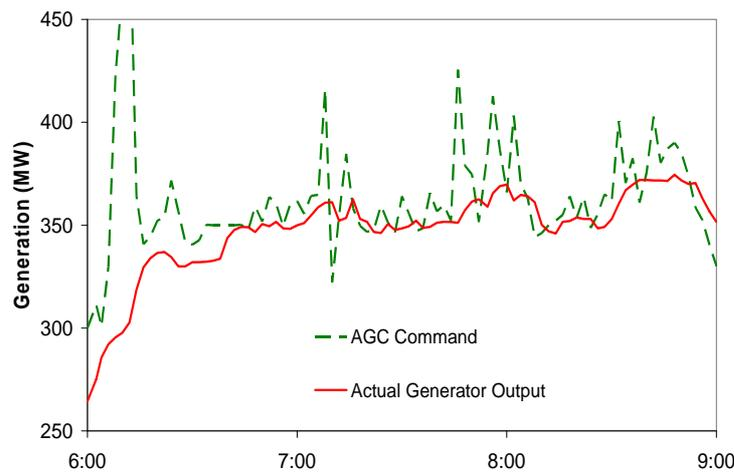
**Figure 4 Conventional turbine generators sometimes follow AGC commands poorly.**
