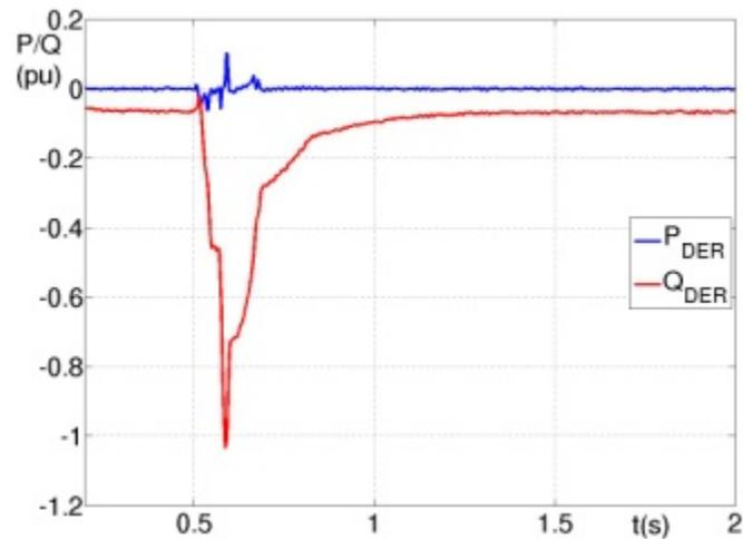
**Figure 9 Local Voltage Support to Prevent a Motor from Entering a Stalled Condition [6]**
