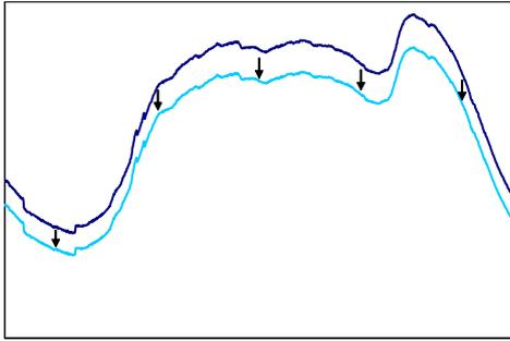
**Figure 5 Morning and Afternoon Peaks in Load With Reduction due to Efficiency**
